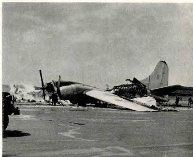
Deviation leads to destruction. Over-torquing was the cause of these.
